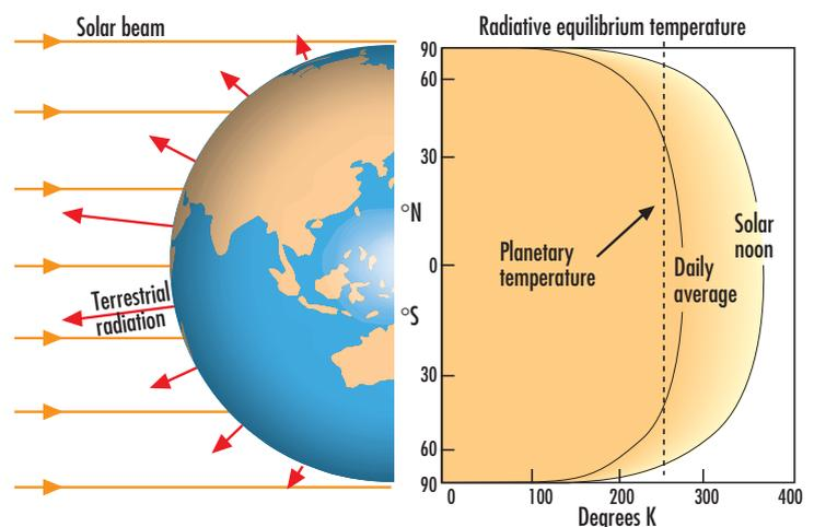
**Figure 2.** A schematic representation of the hypothetical situation of latitude-by-latitude balance between the incoming short wave and outgoing long wave radiation and the resulting north-south radiative equilibrium temperature profiles that would result, at solar noon and as a daily average around the earth, compared with the overall planetary radiative equilibrium temperature of 255K.
