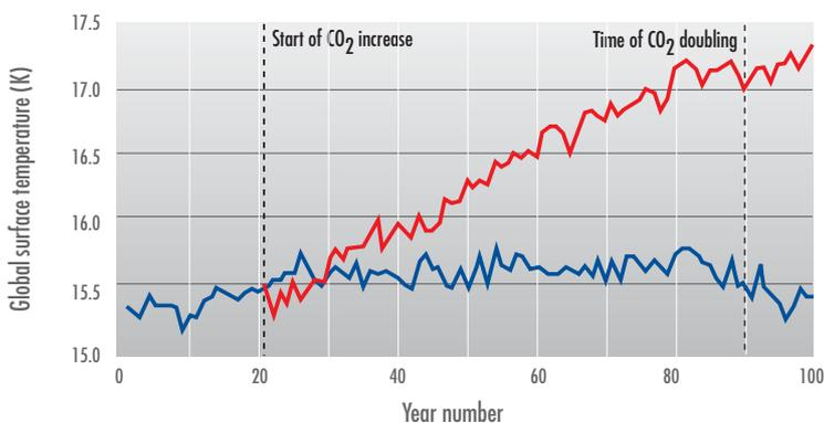
**Figure 60.** Global-mean surface temperature variation with time using the fully-coupled BMRC climate model. The transient run, with CO<sub>2</sub> increasing at 1% per year from year number 29, is compared with a control (1 x CO<sub>2</sub> (330 ppmv)) run.
