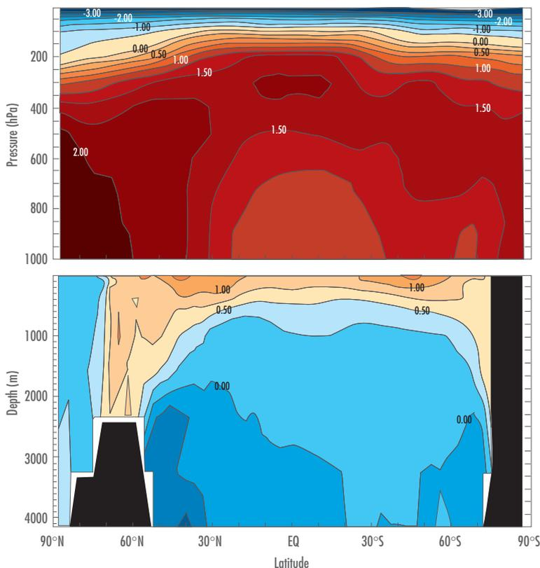
**Figure 63.** A zonal cross-section of temperature changes (transient - control) at the time of doubling in the BMRC coupled climate model. The vertical profile extends from an ocean depth of 4000 m to the surface (OGCM) and from the near surface (1000 hPa level) to the highest modelled level of the atmosphere, above 10 hPa (AGCM).
