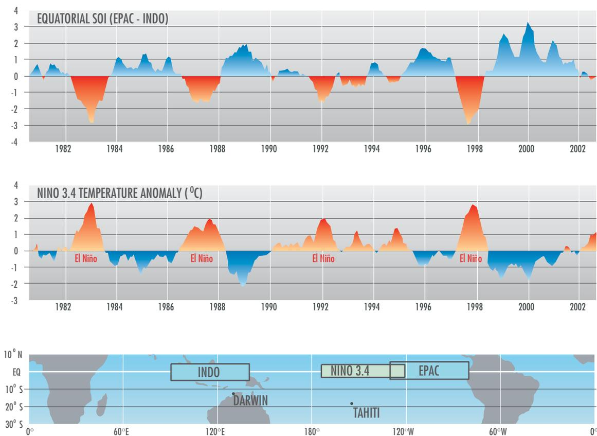
**Figure 46.** The El Niño and the Southern Oscillation from 1980 to 2002. The upper chart shows the variation in equatorial Southern Oscillation Index, a measure of the difference in surface pressure gradients between the Indonesian region (INDO) and the Eastern Pacific (EPAC). The locations of the regions are defined in the lower chart. In the middle is shown the indicative mean temperature anomaly as recorded in the region designated 'NINO 3.4'.
