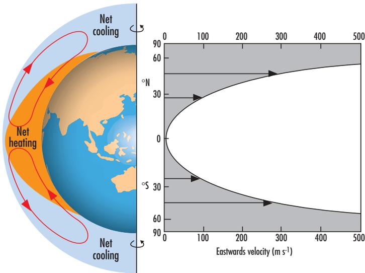
**Figure 10.** The origin of the atmospheric circulation. The strong net heating of the lower tropical atmosphere by sensible and latent heat flux from the solar-heated surface drives the north-south overturning shown schematically on the left. The poleward moving air in the upper atmosphere attempts to conserve the absolute angular momentum it acquired through frictional drag at the surface near the equator and accelerates rapidly eastward relative to the earth's surface as shown on the right.
