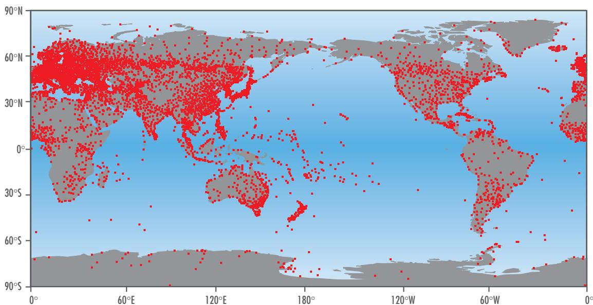
**Figure 30.** The surface synoptic observing network of the WMO World Weather Watch comprises some 3000 stations reporting between two and eight times daily.
