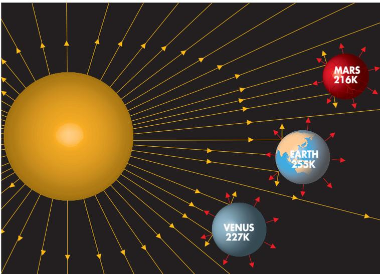
**Figure 1.** The geometry of the sun-earth system and the planetary radiative temperatures of Earth, Venus and Mars. A proportion of the short wave radiation from the sun (orange arrows) is reflected back to space, as determined by the albedo or reflectivity of the planet, but the absorbed short wave radiation heats the planets which in turn radiate long wave energy back to space (red arrows). Sizes and distances are not to scale.
