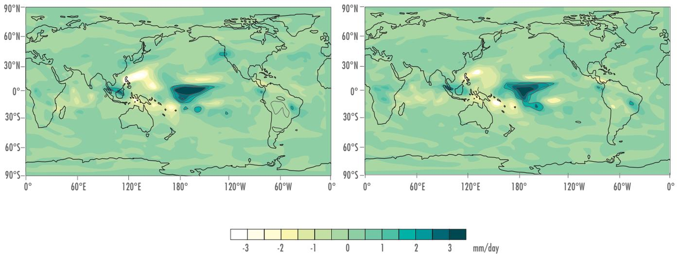
**Figure 64.** Mean December-February rainfall anomalies (mm/day) during El Niño events, in (left) control and (right) transient simulations of a BMRC climate model. The similarity between the rainfall anomaly patterns in this model suggests that greenhouse warming will result in little change to the mean patterns of rainfall anomaly associated with El Niño events.
